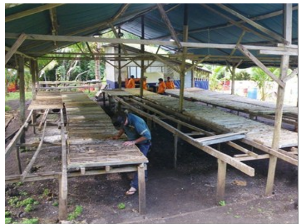
Figure 16: Core Logging and sampling Shed
